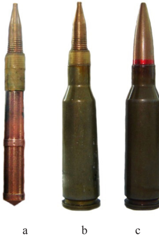
Figure 2.2.27 — The bullet and the cartridge, the 5.45×39PSP: a — bullet cartridge 5,45×39PSP; b — cartridge 5.45=39PSP Assembly; c — cartridge of 5.45×39 (7N6)
