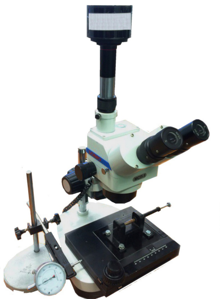
Figure 3.5.1 — General view PAK “BIZAN” for measuring the parameters of traces on bullets and cartridges
