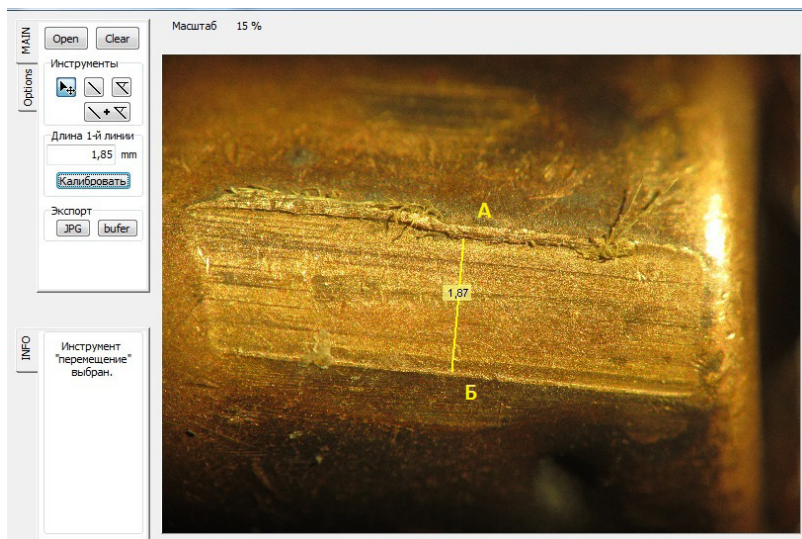
Figure 3.5.4 — The view of the active window of the software application after loading the investigated image of the trace cutting the bore on the surface of the bullet and calibration
