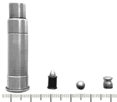
Figure 2.1.1 — General view of the cartridge “Air Cartridge” and the throwing elements used in it [113, pp. 11–18]
