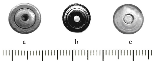
Figure 2.1.4 — General view of the bottom of the holder “Air Cartridge” (a, b) and improvised cartridge (c) represented in the study [113, pp. 11–18]
