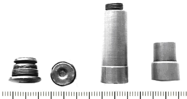
Figure 2.1.3 — General view of the structural elements of the cartridge “Air Cartridge” after dismantling [113, pp. 11–18]
